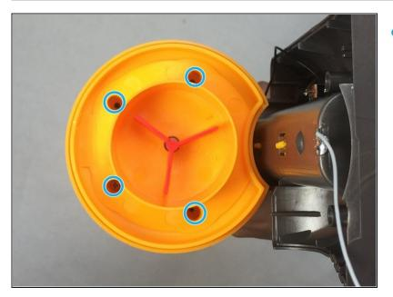
Remove four 9.2mm (0.32 in) screws on bottom of air cylinder motor mount using the PH00 screwdriver.
