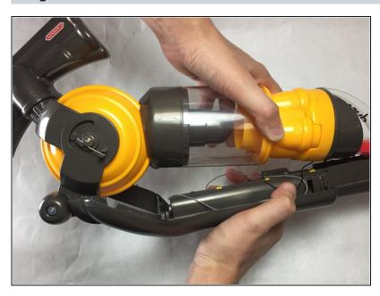
Separate the battery compartment from the ball and bead cylinder by sliding the vacuum ball away from the battery compartment.
