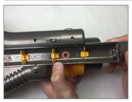
• Remove one 11.5mm (0.45 in) screw in battery compartment using the PH00 screwdriver.
