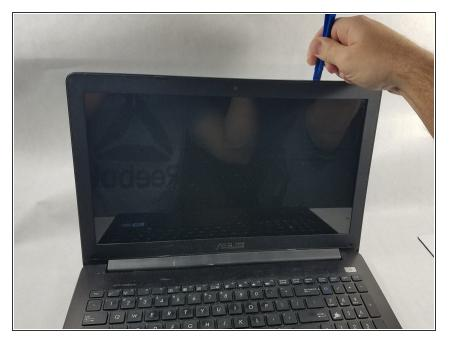
• Using the plastic opening tool, pry the screen frame away from the screen.
