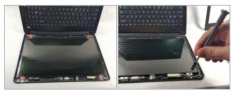
Using the Philips #00 screwdriver, remove the 4 screws holding the laptop screen in place.
