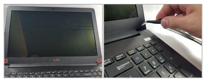
Using the tweezers, remove the 2 black plastic adhesive covers from the bottom corners of the screen frame.
