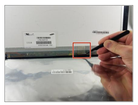
Using the tweezers, peel back the tape securing the screen wire to the laptop.
