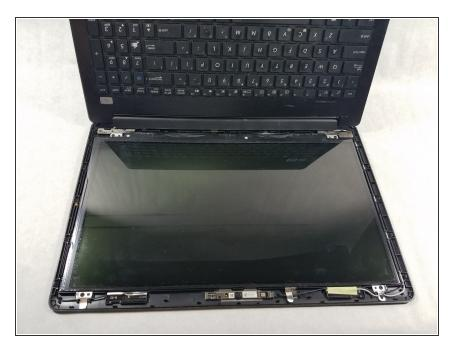
Flip the laptop around and lay the screen flat on your work space with the laptop hinge away from you and the keyboard assembly standing vertical.
