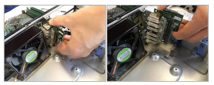
Carefully grasp the audio panel from the sides, pull it back and out of it's slot.
