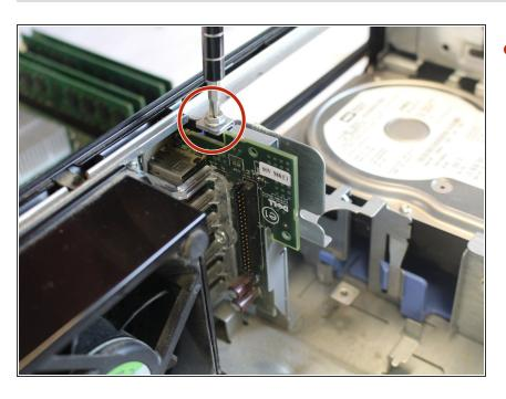
Using a Phillips #2 screw driver, unscrew the 9.5 mm screw that holds the audio panel in place.
