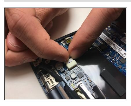
Disconnect the charging port from the motherboard by gently tugging on the plastic part of the connection.
