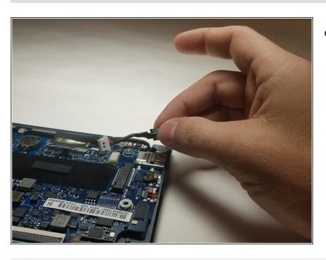
Remove the disconnected charger port.
