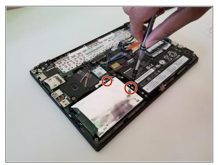
• Remove the Hard Disk Drive card by screwing the 2 0.2mm Phillips screw
