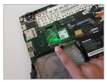
• Take off the connector by carefully popping its holders out of place
