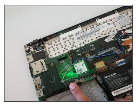
• place the connector in order to hold the cable
