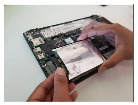
Reconnect the cable to the new Hard Disk Drive
