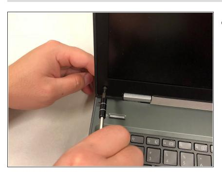
Use a T9 screwdriver to unscrew both 0.4mm Torx screws.
