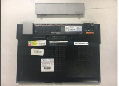
Remove battery by sliding the locks inward and pushing the battery out.
