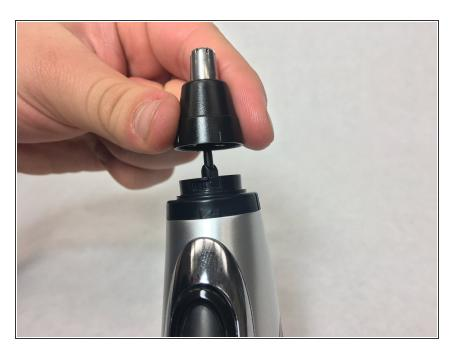
Rotate the blade block counterclockwise and remove.
