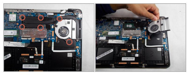
• Using a Phillips #0 screwdriver remove the six screws holding the CPU Fan and Heatsink in place.
