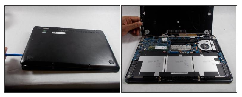
• Carefully remove the backplate using the plastic opening tool.
