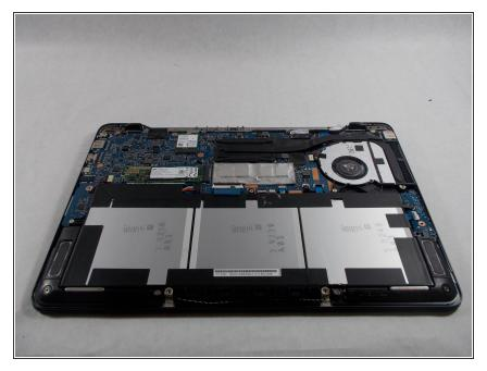
• Locate the battery near the bottom.
