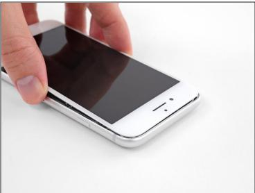
• Slide the display assembly slightly down (away from the top edge of the phone) to disengage the clips holding it to the rear case.
