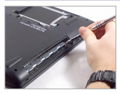
Start by unplugging the laptop and turning it upside down. There are 3 screws in the disk drive, remove those using a Phillips #0 screwdriver.
