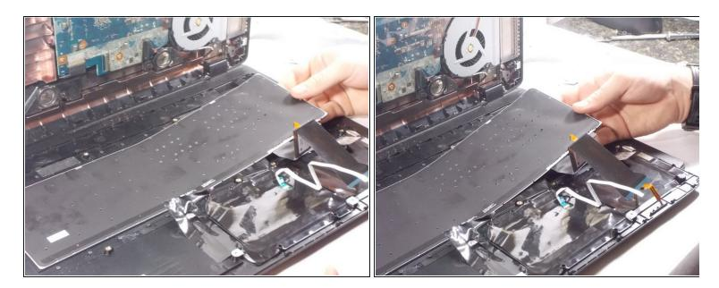
• Lift up the keyboard panel and replace it with the new one.
