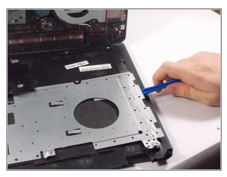
Gently take off the metal keyboard cover by using the blue opening tool.
