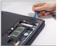
• Use the blue opening tool to gently separate the back panel by loosening it on all sides to ease the outer shell of the laptop until it separates.
