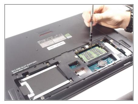
Remove the medium sized panel attached on the back. Then using your Phillips #0 screwdriver, remove all 8 screws.
