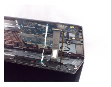
Gently lift the outer shell up until the white, gold and silver power strips are visible. Proceed by removing the strips from the bottom side of the keyboard. Finish removing the outer shell.
