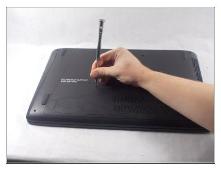
Unscrew both 8mm phillip's head screws that hold on the access gate.
