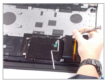
Remove the two Phillips #0 screws located on the panel above the white power strip.
