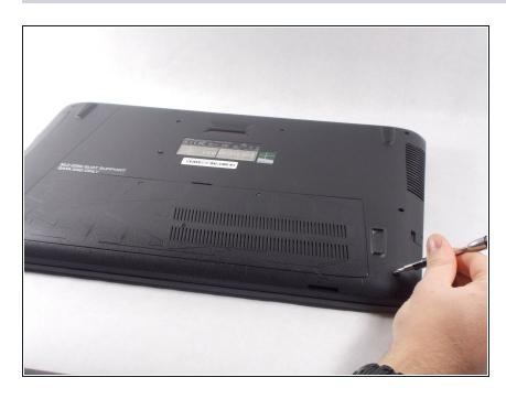
Remove the entire large back panel (outer shell) by removing the screws closer to the outer edge.
