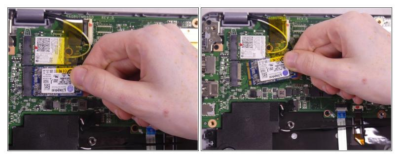
Remove the SSD card from the motherboard by gently pulling up on the side where the screw originally was and out in the same direction.
