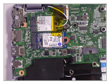
• Remove the Phillips 3.6 mm screw using a Phillips #1 screwdriver.
