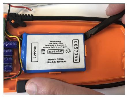
• Using the spudger, pry the battery off the back cover.
