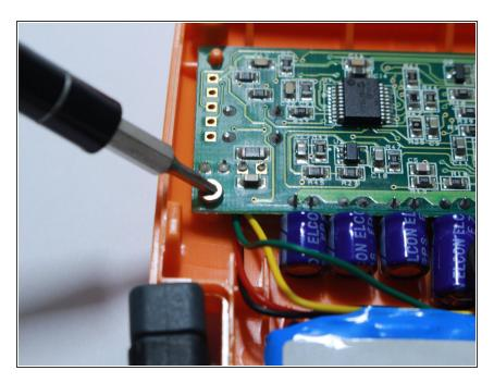
Using a T6 Torx screwdriver, unscrew the 5.66 mm screws attaching the circuit board to the case and flip the circuit board.
