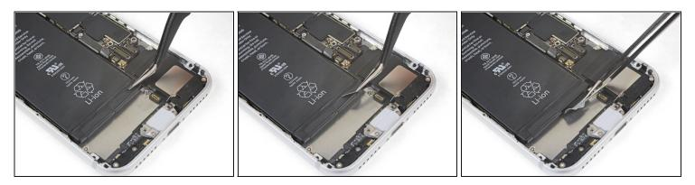
Peel back the first battery adhesive tab from the bottom right edge of the battery.
