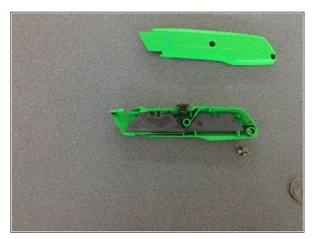
Carefully pull up on the top half of the cutter exposing the blade on the inside.
