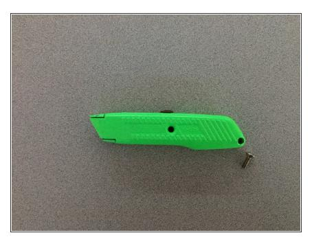
Using a screwdriver or a coin remove the single screw in the center of the box cutter
