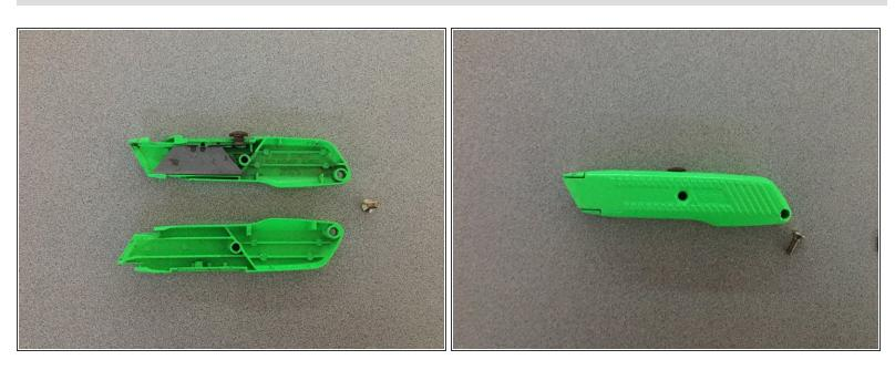
• With the fresh blade in place carefully place the upper half of the box cutter on the lower half that contains the blade as shown in image number 2.
