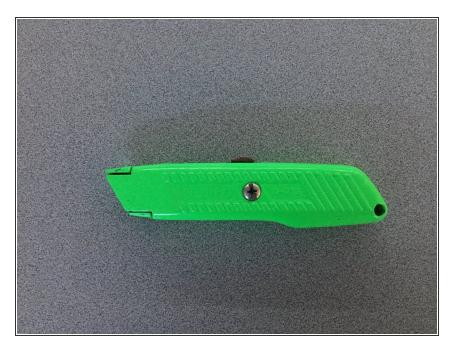
With the center screw re-installed you are all set to use your Stanley 10-079 box cutter again with a brand new blade.
