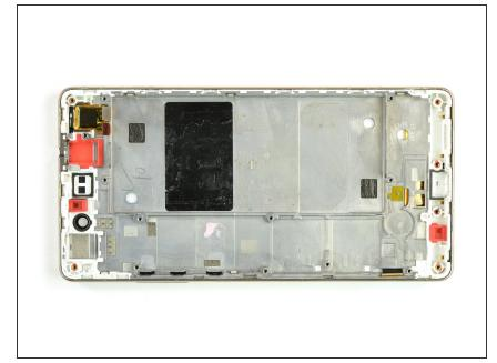
Inspect your **new** display assembly and be sure to transfer any missing parts from the old one.
