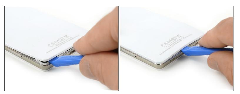
Use an Opening Tool and start to lever up the back cover of your Huawei P8 Lite at the bottom of your phone.
