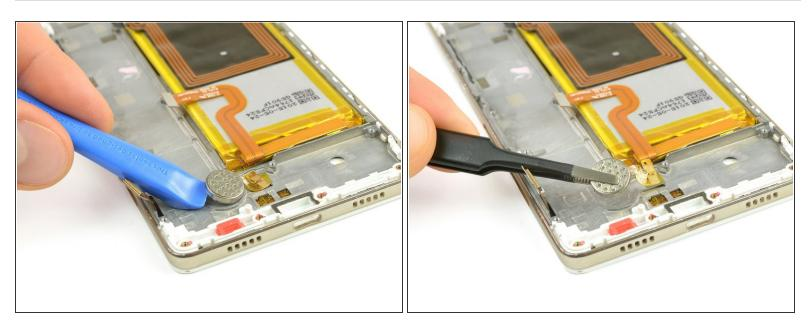
Pry off the vibrator using a plastic opening tool.
