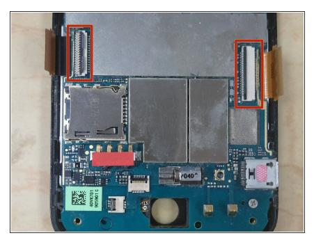
Use your spudger to release the remaining clips, disconnecting the ribbon cables from the logic board.
