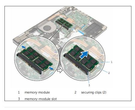
• Remove the memory module from the memory-module slot.
