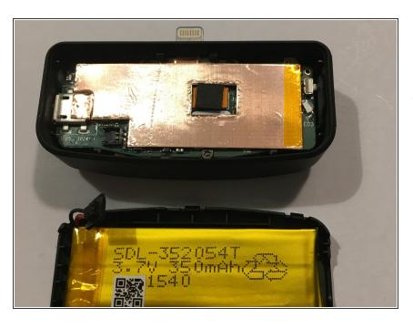
The two halves will separate very easily and the battery connector will detach very easily.
