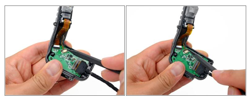
Use the tip of a spudger to push out the retaining clip on the viewfinder backlight ribbon cable ZIF connector.
