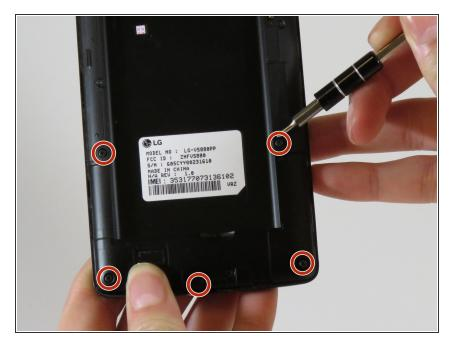
• Use a Phillips #000 screwdriver to remove five 3.0 mm screws.
