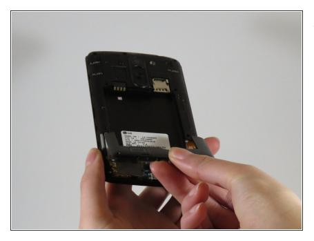
To insert your new loudspeaker, simply take the piece and snap firmly into the place of the previous loudspeaker.
