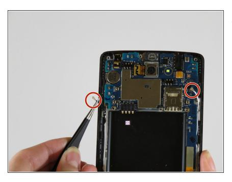
Use a pair of tweezers to lift up the white antenna wire. On the other side of the logic board, do the same for the black antenna wire.
