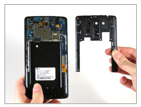
Remove the hard shell covering the motherboard.
