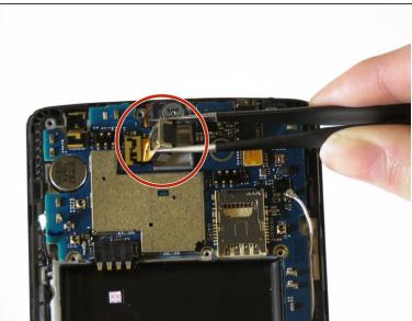
Use the tweezers to remove the four connectors as well as the back camera.
