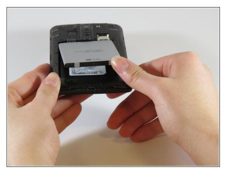
Lift the battery out of its place by prying up from the small notch at the base of the battery.
