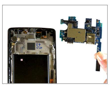
Lift up and remove the motherboard from the device. To reassemble your device, follow these instructions in reverse order.
