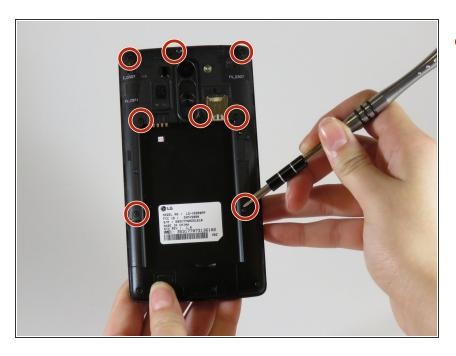
Remove the eight 3.0 mm screws using the Phillips #000 screwdriver.
