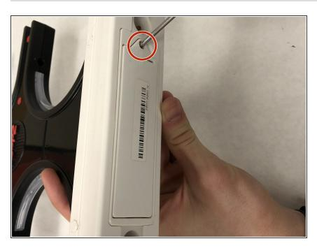
Use a No. 2 Phillips head screwdriver to take out the 1/4" screw that holds the battery cover in place on the bottom of the device.
