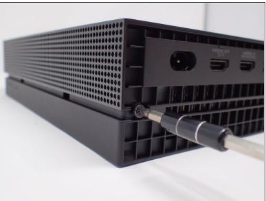
Use a T9 Torx screwdriver to remove the 13mm screw which is under and to the left of the power input.
