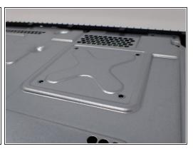
Using a T9 Torx screwdriver, remove the four 9mm screws that are holding the heat sink to the outer metal casing.
