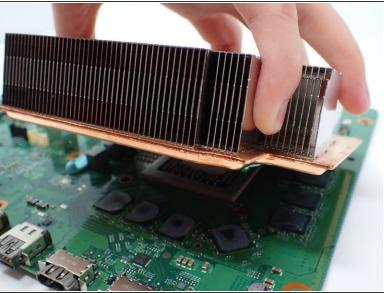
Lift the heat sink to detach it from the motherboard.
