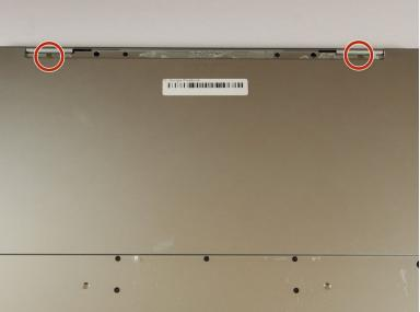
Remove the two yellow 2.0mm screws by using a T3 Torx screwdriver.
