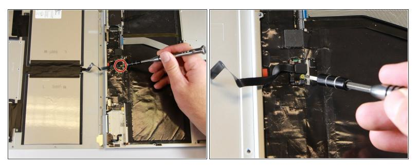
Remove the yellow 2.0mm screw from the middle of the panel by using the T3 Torx screwdriver to turn the screw counterclockwise.
