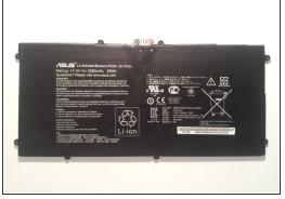
To remove the battery, remove the 8 screws then work your spudger underneath the battery between the 2 cells to work it free of the adhesive that fastens it to the case.
