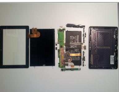
With the LCD free, you should now be able to lay it out in a big pile of parts and the teardown is complete. Now let's see what's under all those heatsinks and tape.
