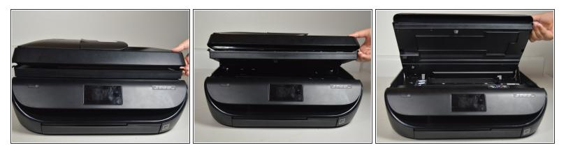
Open the cartridge access door by using putting one hand on the grooves of each side and pulling up.
