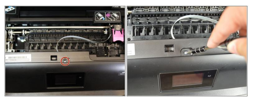
Using the 2.0mm screwdriver, remove the 14mm hex screw that binds the front cover to the printer body by turning the screw counterclockwise.
