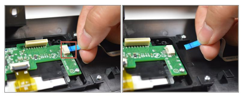
Remove the other connector that is attached to the screen's circuit board by pinching the blue part
