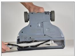
Slide the roller belt off of the roller brush and pull the roller away from the motorized brush.
