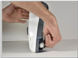
Use the bristles to pull the end of the brush that was connected to the belt away from the vacuum.
