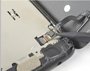
Slide the point of a spudger underneath the fingerprint sensor cable and gently pry up to loosen the cable from the phone.
