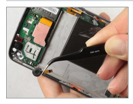
Pry the vibrator motor from its position.
