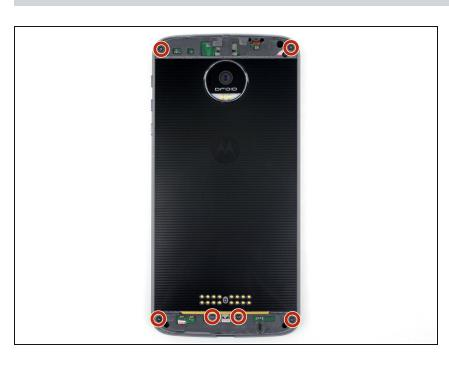
Remove the six 4 mm T3 Torx screws securing the display assembly.
