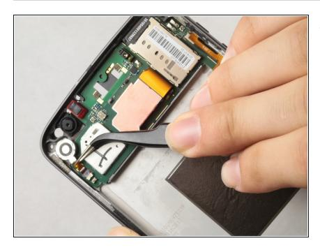
Use tweezers to flip open the ZIF connector and remove the vibrator ribbon cable.
