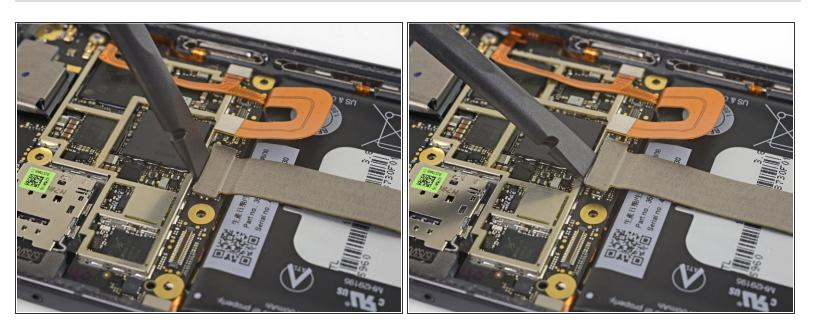
Use the flat end of a spudger to disconnect the charging assembly connector.
