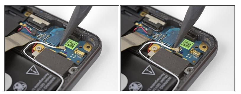
Use the point of a spudger to pry the white antenna cable connector straight up and disconnect it from the charging assembly board.
