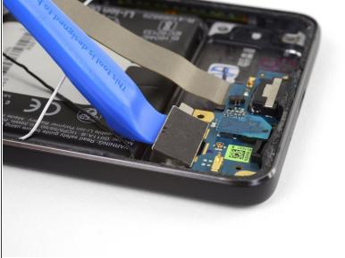
• Use an opening tool the gently lift the vibration motor and separate it from the adhesive holding it to the phone.
