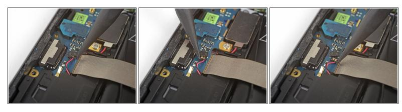
Use the tip of a spudger to gently push the speaker cable connector out of its socket horizontally, alternating pushing either side of the connector out a little bit at a time.
