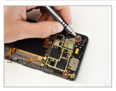
Remove the two 2.5 mm PH00 screws.
