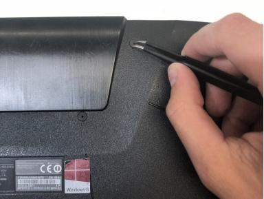
Use a pair of tweezers to remove the top four rubber stoppers found on the bottom of the laptop.
