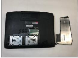
Use the nylon spudger to remove the back center panel.
