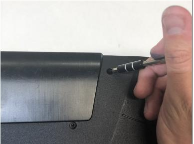
Use a Phillips 1 Screwdriver to remove the top four 8.5 mm screws.
