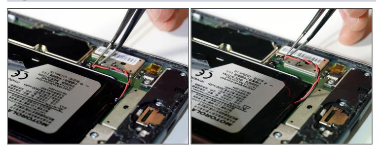
• Detach the red and black battery wire by lifting up with tweezers.
