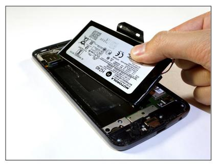
• Lift to remove the battery from the device completely.
