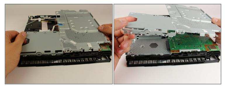
• Remove the metal plate by grabbing two sides of the plate and lifting up and away from yourself.
