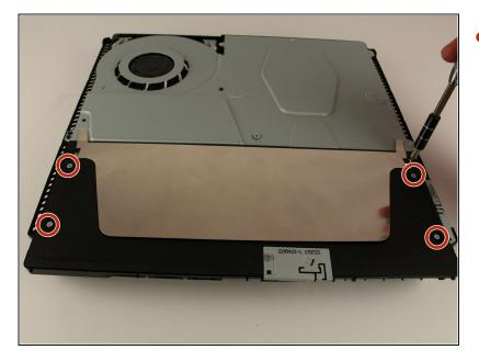
Remove the four 16mm Philips screws holding the power supply in place.
