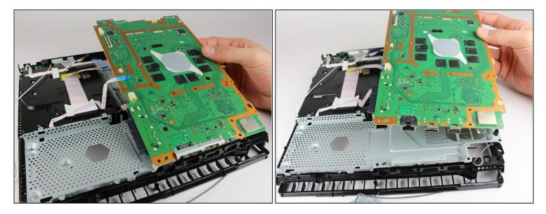
• Remove the motherboard by grabbing the edge of the board with one or two hands and pulling away and up.
