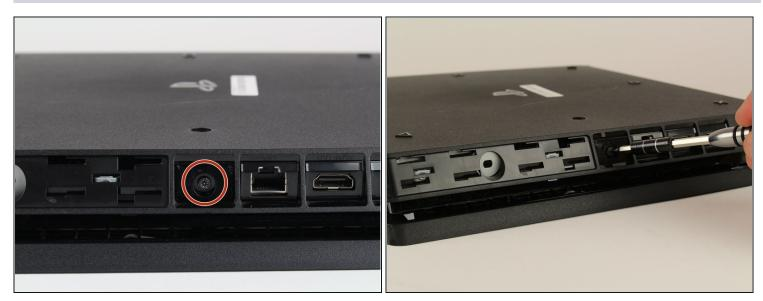
• Unscrew and remove the now exposed 5.0mm screw using a T8 security Torx screwdriver with a counter-clockwise motion.
