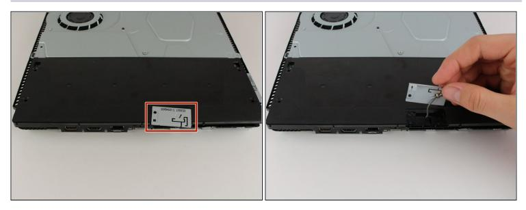
• Remove the antenna from the top of the power supply by guiding the wire with your fingers through the groves underneath the metal panel.
