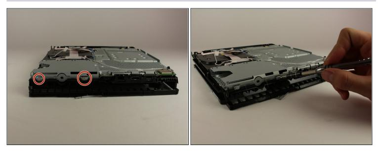
Unscrew and remove the two 5.0mm screws on the side of the console using a Phillips #1 screwdriver with a counter-clockwise motion.
