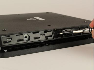
• Unscrew and remove the 5.0mm screw that was behind the sticker using a T8 security Torx screwdriver with a counter-clockwise motion.
