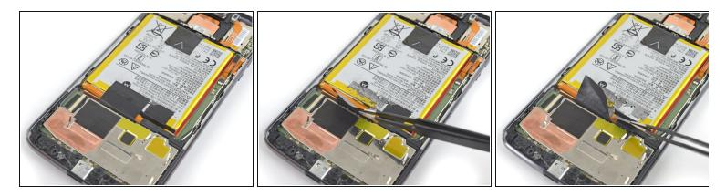
• Use a pair of tweezers to remove the two black pieces of tape securing the battery.
