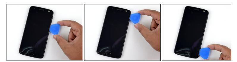
Slide your opening pick all along the right side of the device to release the clips and adhesive securing the screen assembly.
