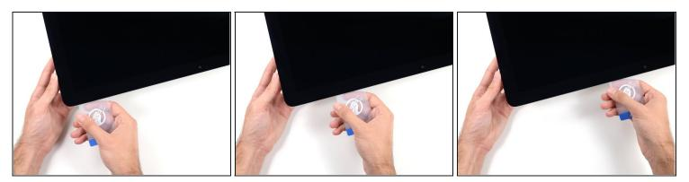
• Slide the card toward the center of the display to cut any of the remaining adhesive along the top right corner of the iMac.
