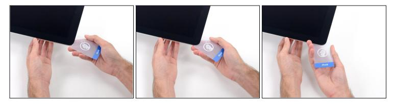
• Insert a second plastic card into the gap between the display and frame near the top left corner of the iMac.
