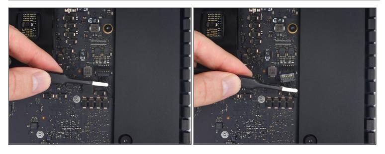
• Gently pull the right speaker cable connector parallel to the logic board, straight out of its socket on the logic board.
