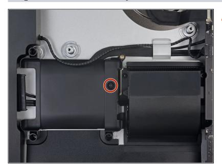
• Remove the 7.3 mm T8 Torx screw securing the hard drive tray to the rear enclosure.
