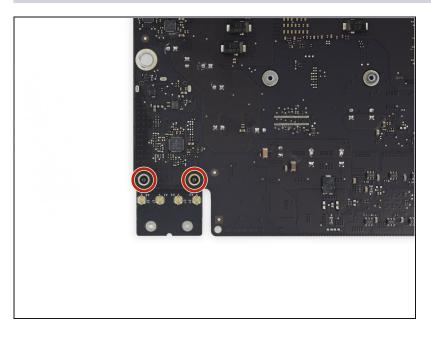
• Remove the two 3.3 mm T5 Torx screws securing the AirPort/Bluetooth card to the logic board.
