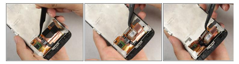
• Lift the digitizer wiring with a pair of tweezers but do not pull out the wiring.
