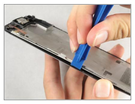
• Begin to separate the front screen from the metal plate with the plastic opening tool.
