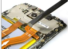
Use the flat end of a spudger to disconnect the display, daughterboard interconnect, and battery cables.
