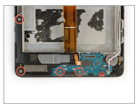
Remove the four Phillips #00 screws holding the daughterboard and loudspeaker to the phone.
