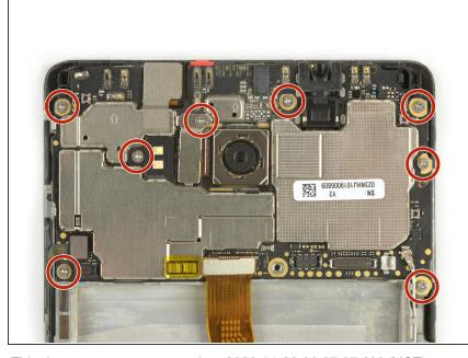
Remove the eight Phillips #00 screws securing the motherboard to the phone.
