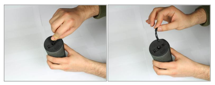
• After the D-ring has been removed, the rubber port cover can be removed.
