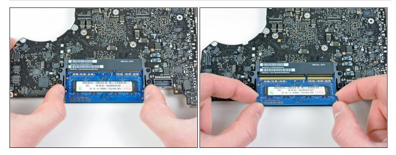
• Pull the two RAM retaining arms away from the center of the RAM chip.
