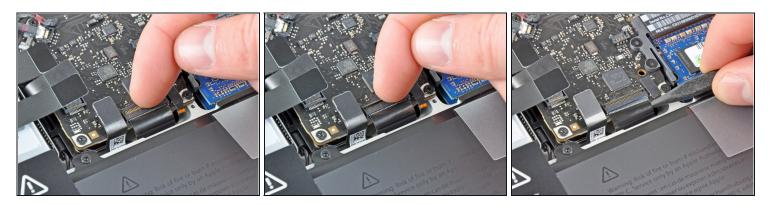
• Use your fingernail to flip up the retaining flap on the keyboard ribbon cable ZIF socket.
