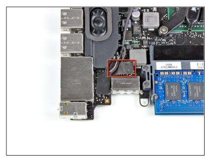
• Remove the small piece of black tape covering the left speaker connector.
