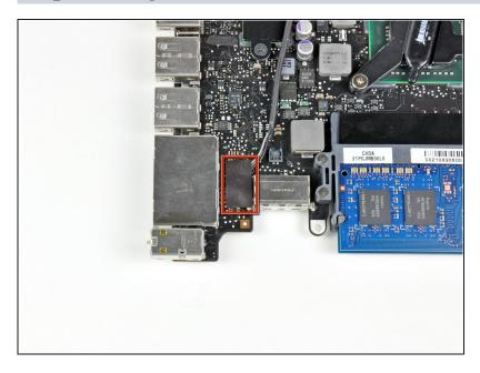
• Remove the piece of black tape covering the microphone connector.
