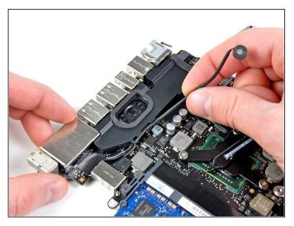
• De-route the microphone cable from its slot molded into the left speaker enclosure.
