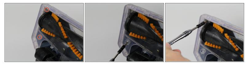
• Remove screws from the left side of the white plastic frame.
