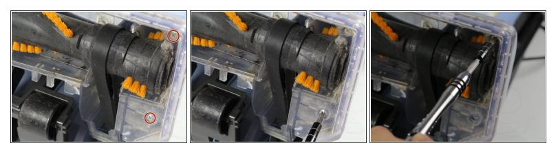
• Use a Phillips #1 screwdriver to remove the screws from the right side of the white plastic frame.
