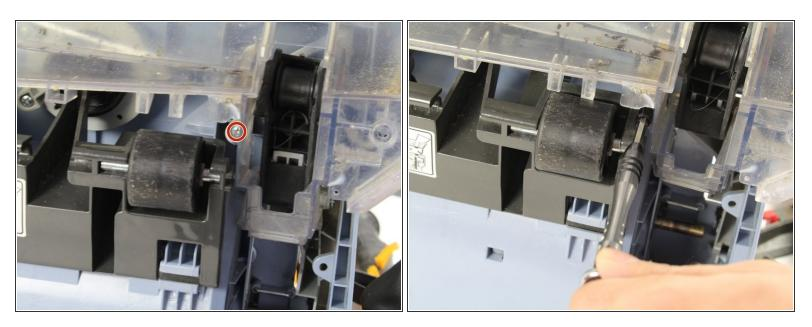
Remove the screws at the bottom of the white frame near the roller.
