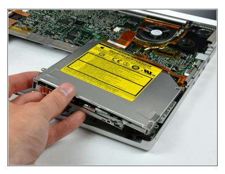
Lift the optical drive out of the lower case, being careful not to disturb the PRAM battery & USB board ribbon cable.
