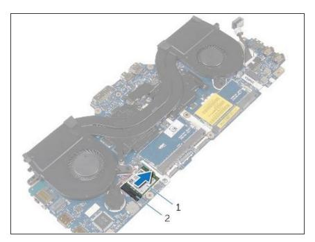
Slide the wireless NEW card into the wireless-card slot on the system board.
