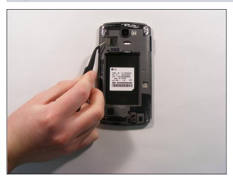
Using <u>Tweezers</u> grab onto the Micro SD Card and remove.
