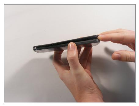
• Insert fingernail into the slot on the back left side of the phone and pry open.
