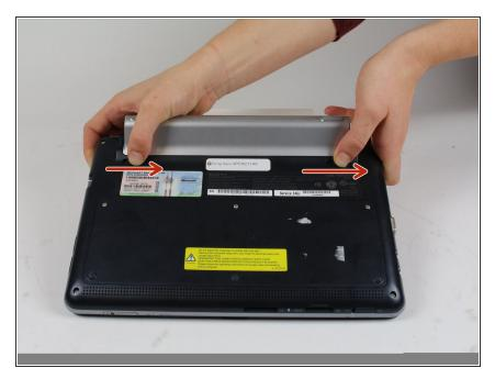
Place your hands on the lock/unlock function on the laptop on either side on the bottom of the laptop and slide.
