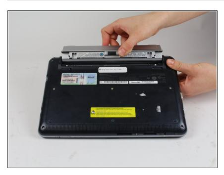
Carefully remove the battery from it's slot
