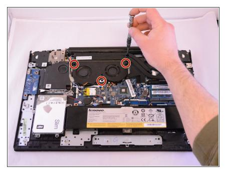
Using the Phillips #0 screwdriver, remove the three screws connecting the fan to the device.
